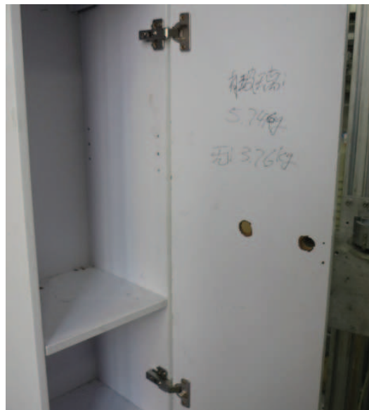
Pic. 2: Hinge mounted with a door (1)
